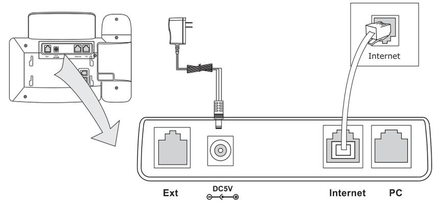
**Note:** If inline Power (PoE ) is provided, do not install the AC adapter. Make sure the Ethernet cable and switch/hub are PoE compliant.
